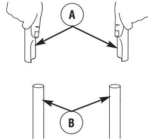
**NOTICE** It may be necessary to move the handle supports from side to side in order to align the handle so it will slide over the handle supports.
