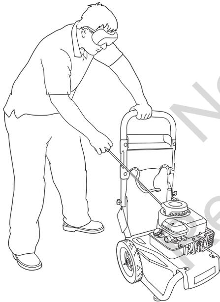
**▲ WARNING** Starter cord kickback (rapid retraction) will pull hand and arm toward engine faster than you can let go which could cause broken bones, fractures, bruises, or sprains resulting in serious injury.
