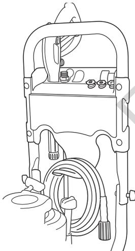
2. Place spray gun through hole on accessory tray on right side of unit.
