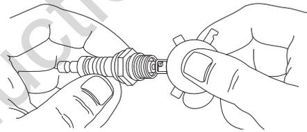
5. Install spark plug and tighten firmly.
