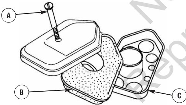
2. Carefully remove air cleaner assembly to prevent debris from falling into carburetor.
